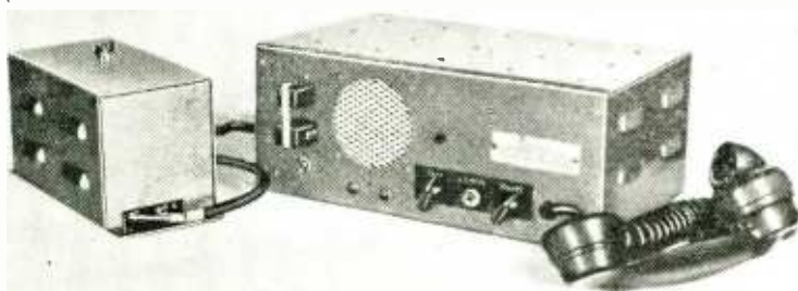
Hudson v.h.f. mobile radio-telephone installation. The unit on the left is the power supply.
