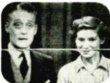
Characteristic interference patterns produced on a television receiver by a nearby 60-watt vacuum (traction type) lamp.
