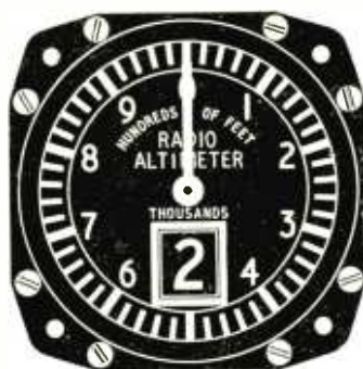
Fig. 5. Face of the height indicator. The full scale represents 1,000 ft, so the pointer makes five revolutions for 5,000 ft. Integral thousands are clocked-up in the window at the bottom.
